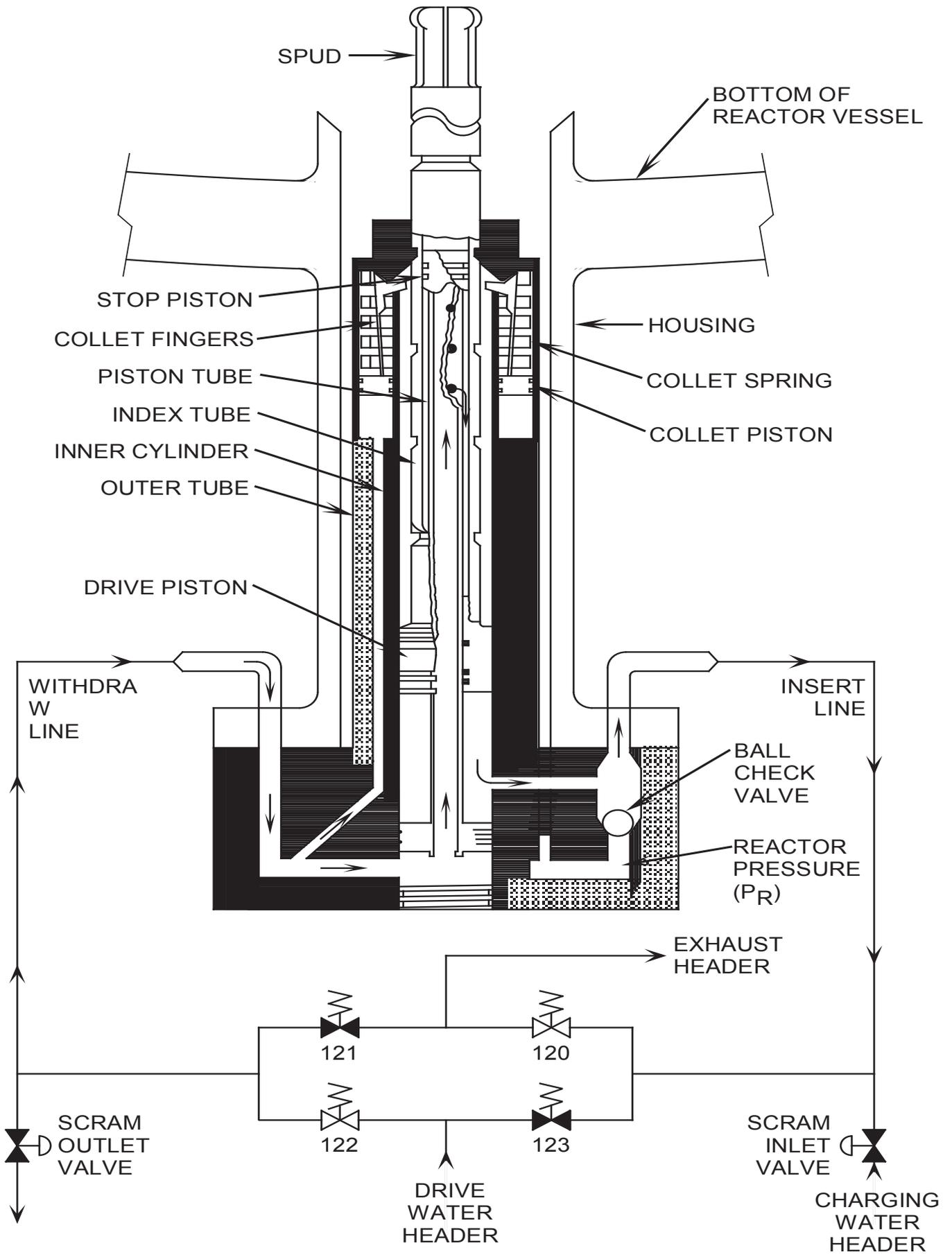
Figure 2.3-11 CRDM Operation (Withdraw)
