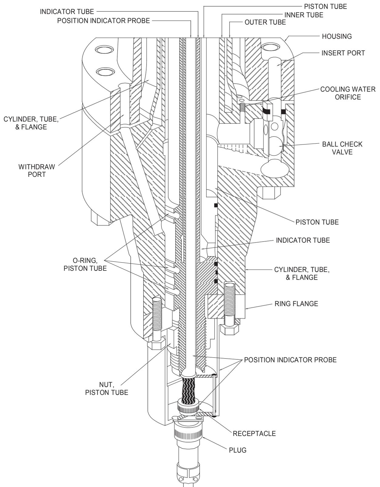
**Figure 2.3-5 Enlarged Cutaway of Lower CRD**
