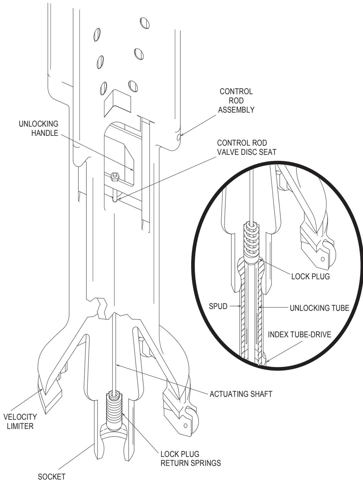
Figure 2.3-6 Control Rod Velocity Limiter and Coupling Mechanism
