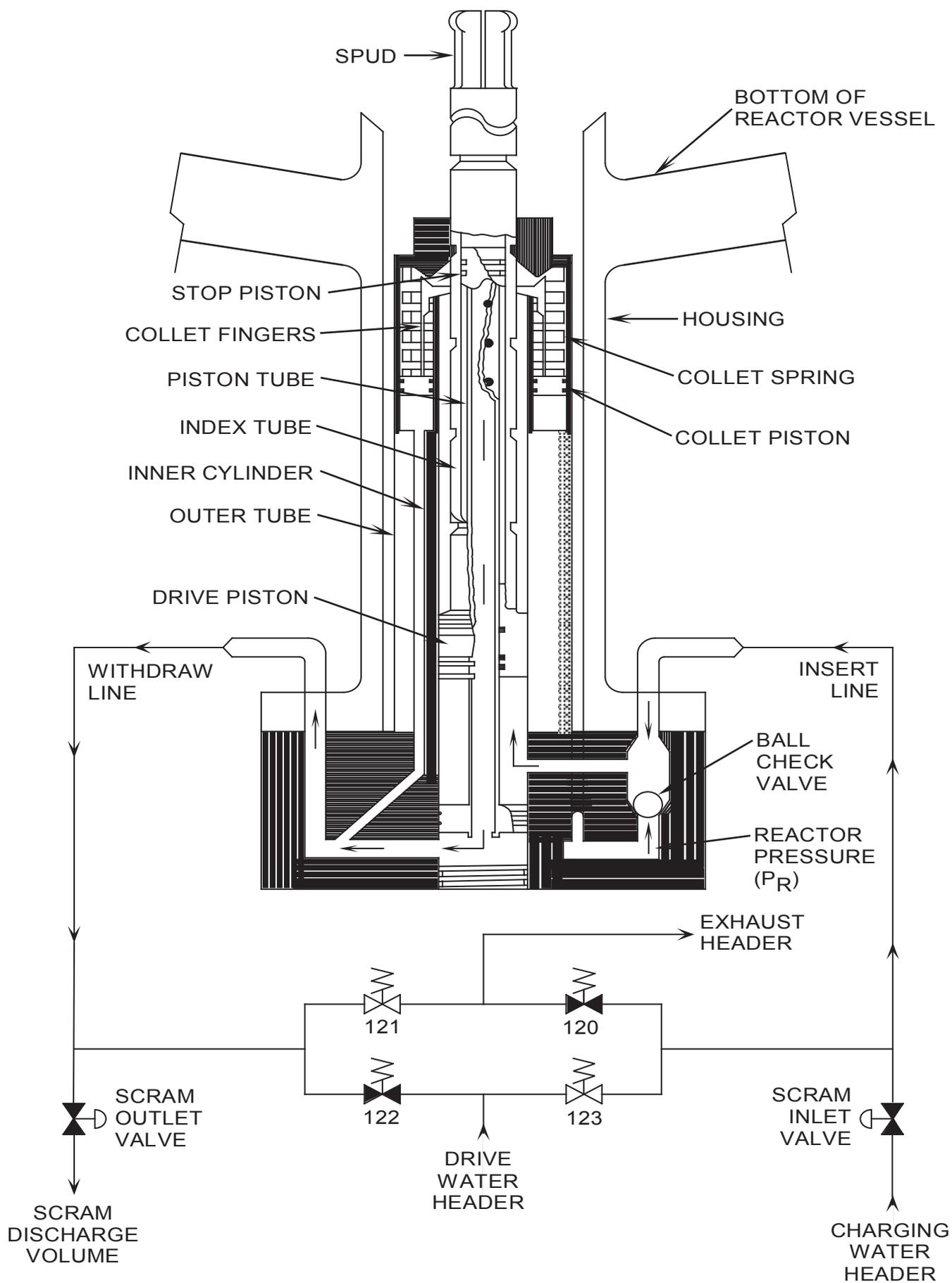
Figure 2.3-9 CRDM Operation (Insert)
