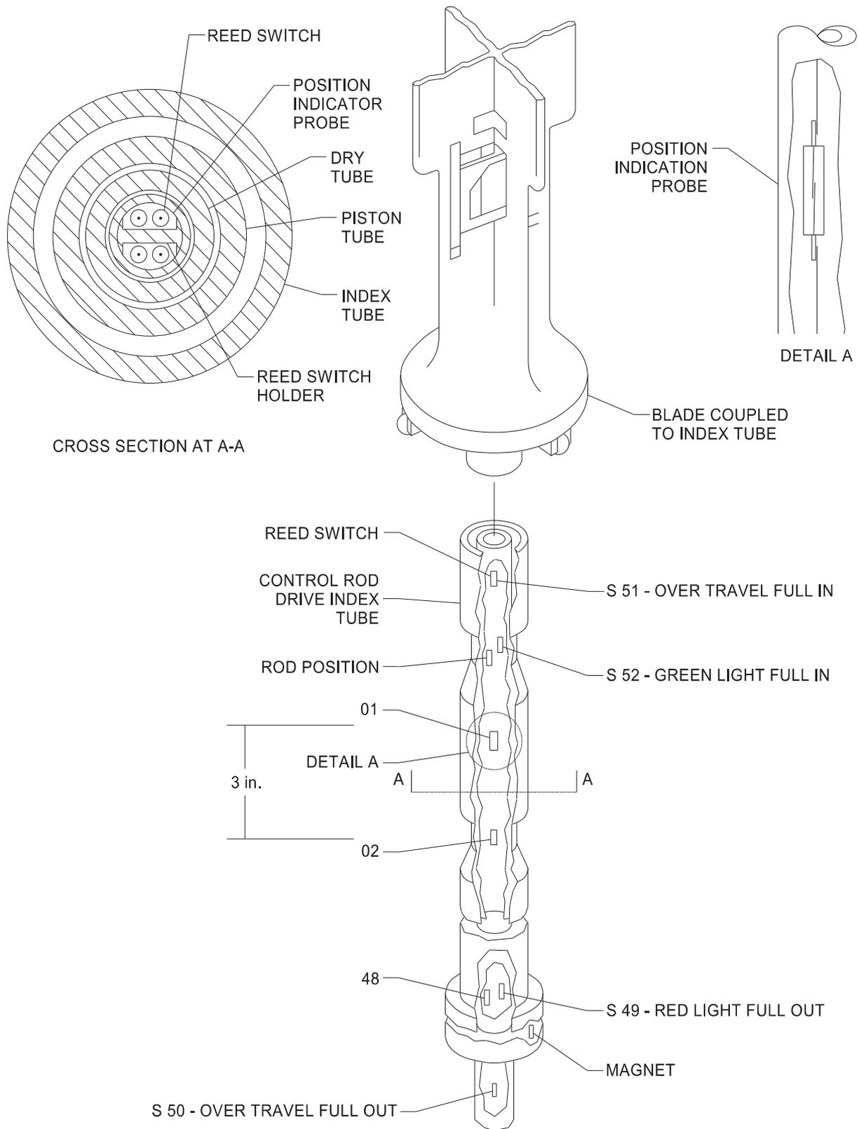
Figure 2.3-7 Control Rod Position Indication
