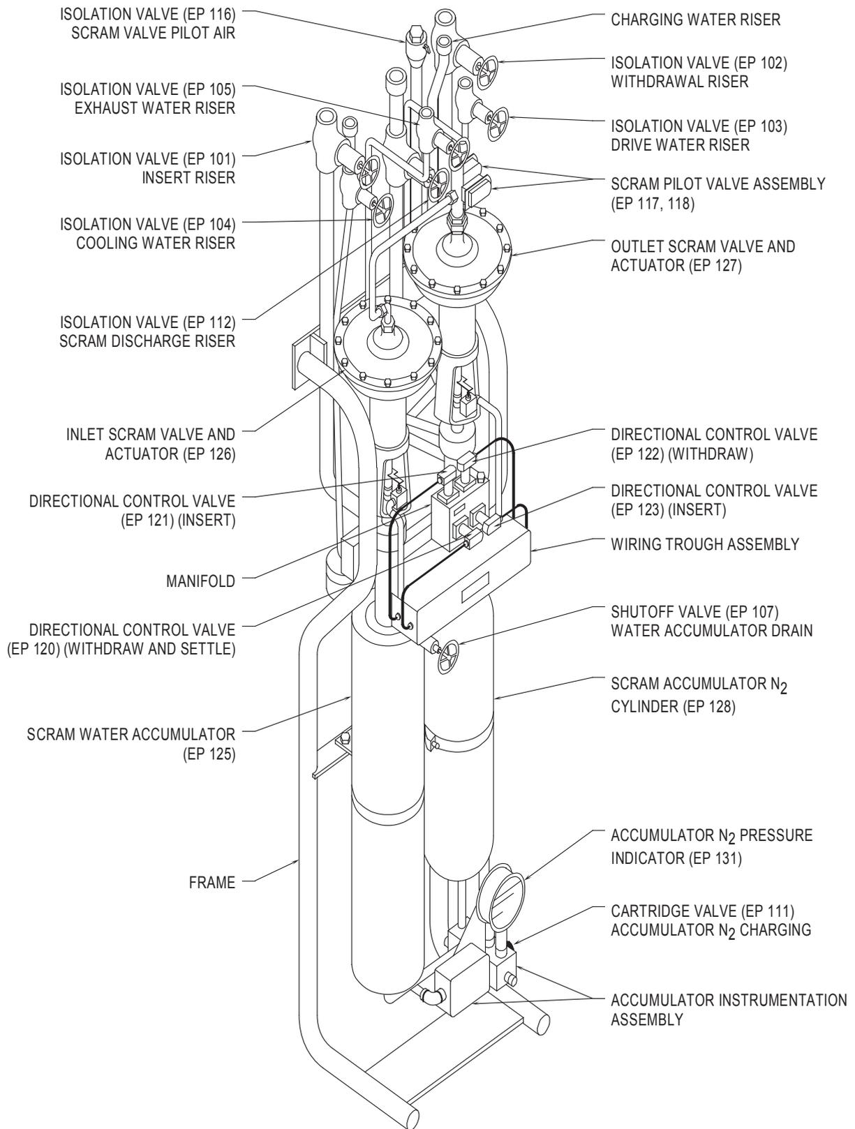
**Figure 2.3-2 Hydraulic Control Unit**
