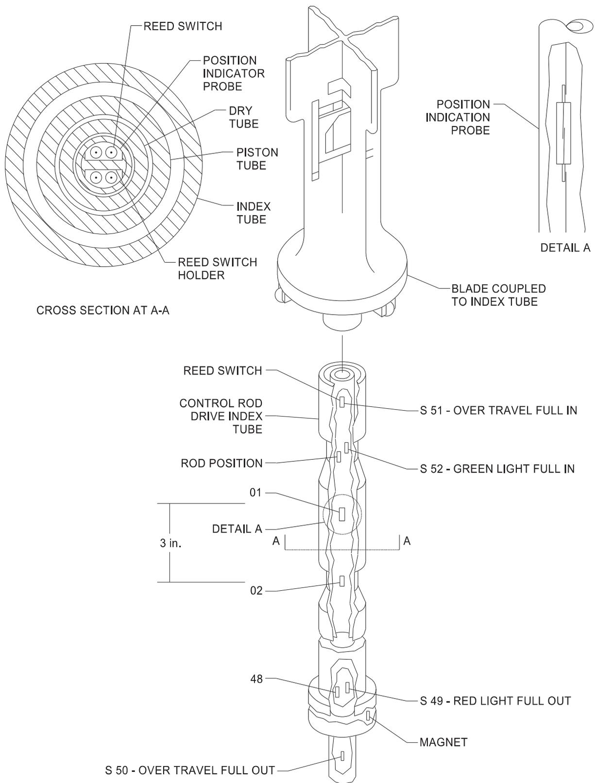
**Figure 2.3-7 Control Rod Position Indication**
